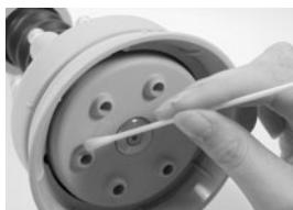
*Only* use diluted (2%) non-toxic quaternary ammonium salt disinfectant or diluted (1%) sodium hypochlorite solution. Use a swab to clean underside of dispenser and ejection holes.
